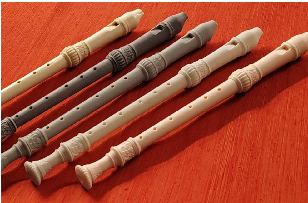
Figure 4: Prints of the Denner RCM0063 recorder in various materials. From left to right: the original instrument; MJF Nylon-12, sanded; grey MSLA resin; SLS glass-filled Nylon-12; MSLA ceramic-resin composite. Photo: G. Rossi Rognoni
