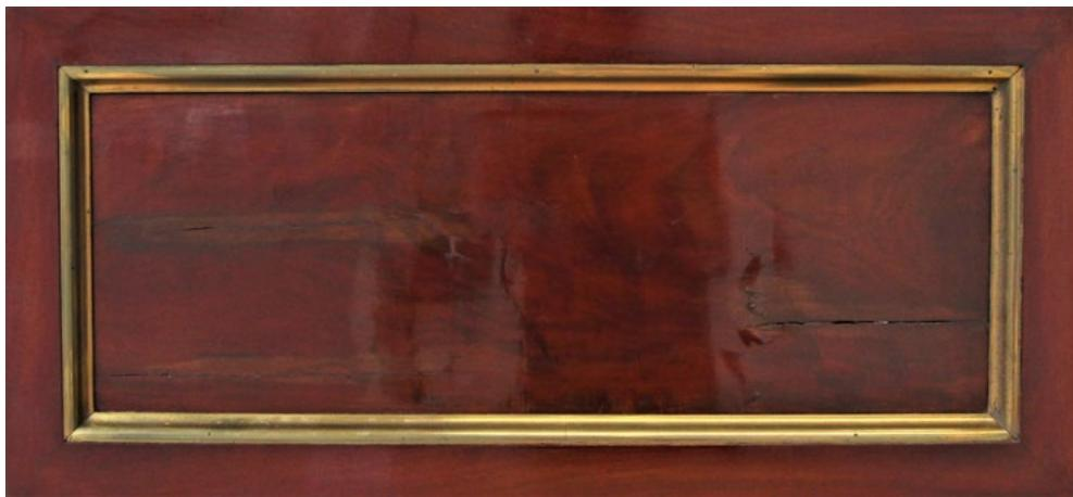
Figure 2: One of the panels (rotated) with the cracks, blistering veneer and discolourations. Photo: Tirza Mol
