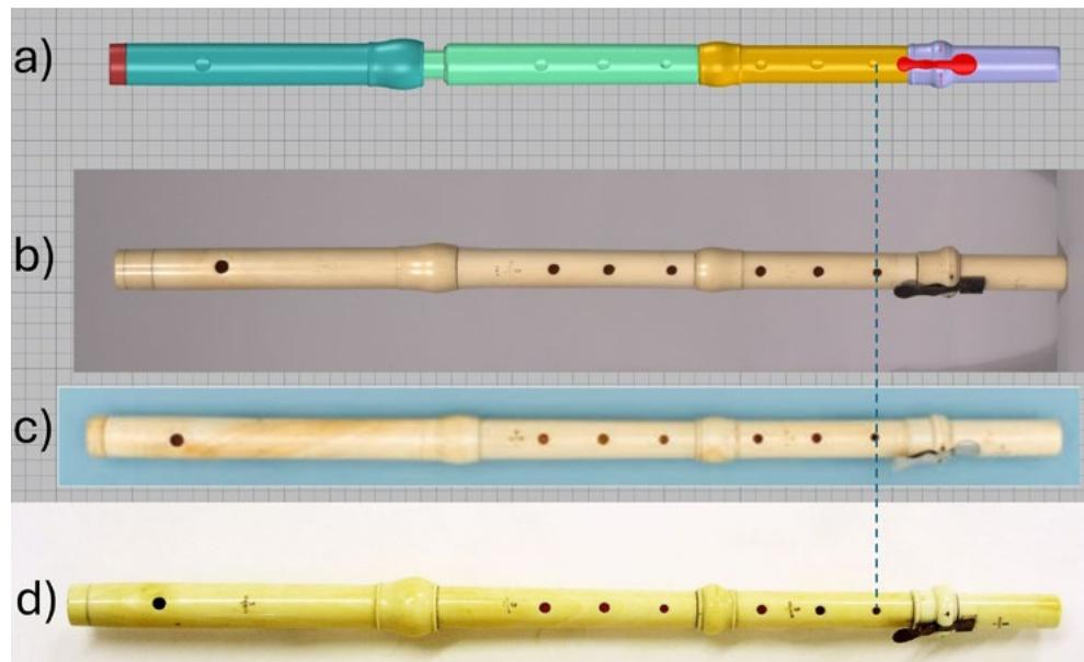
The scanning of each instrument required approximately 6–10 hours, often having to take multiple scans of smaller portions of each piece, which were then ‘stitched’ together, in order to reach a satisfactory definition.
