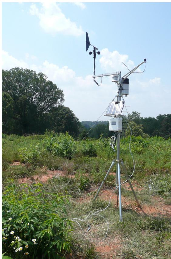
**FIGURE 7.3.** A communicating data logger, solar power panel, and weather sensors. Photo: Michael C. Henry
